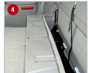
The DU-HA bolts to rear floor flaps to allow access to jack when tilted forward.
